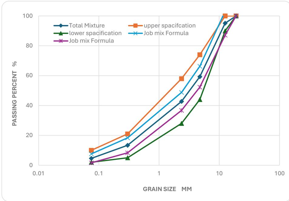
Figure (2): The aggregate's grain size distribution
