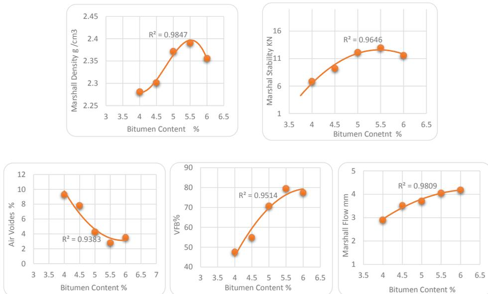
Figure (8): Marshall Test Results for control mix
