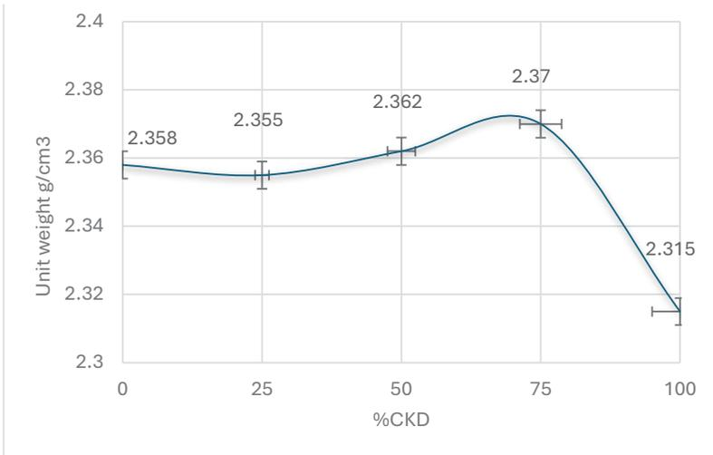
Figure (11): The Effect of CKD on Marshall Unit Weight at (OAC)
