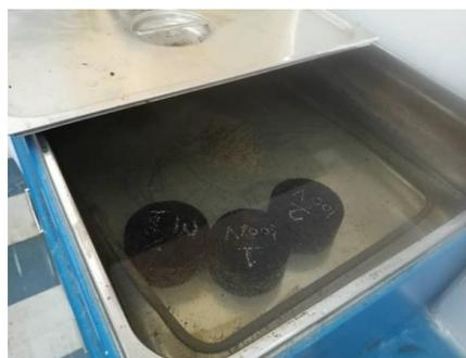
Figure 7: Water Path for Marshall Specimens
