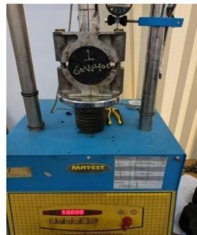
Figure (6): Samples of asphalt concrete for tests of Marshall stability
