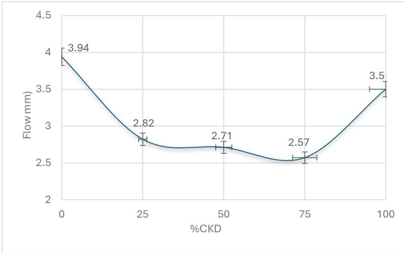
Figure (10): The Effect of CKD on Marshall Flow at (OAC)
