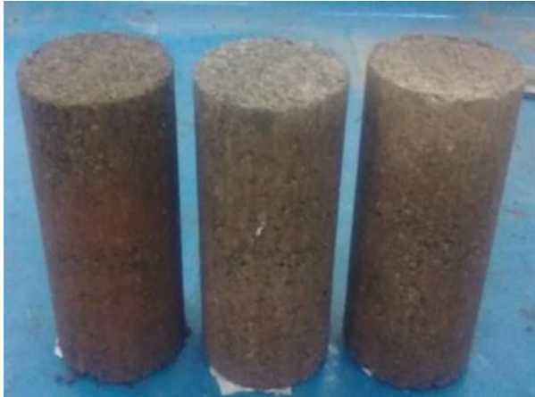
Figure 3: GVA-cement-fine soil samples for UCS, ITS, durability, and UPV tests
